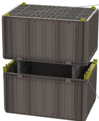
Spacers (Used only with the 330 height AutoStore Bins) – fit along the top edge of the Bins. Must be removed and returned in the bulk container provided.
